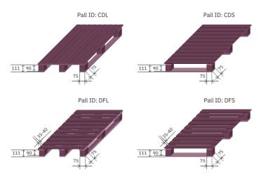
The most frequent pallet types for sheet deliveries used by Holmen Board and Paper.
