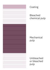
FBB, cream back, is made from layers of mechanical pulp sandwiched between layers of bleached chemical pulp.
