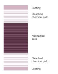
Folding Box Board (FBB, GC1) White back, multiply construction, Incada
