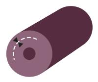
Reel joins are marked by two arrows, above and below each join.
